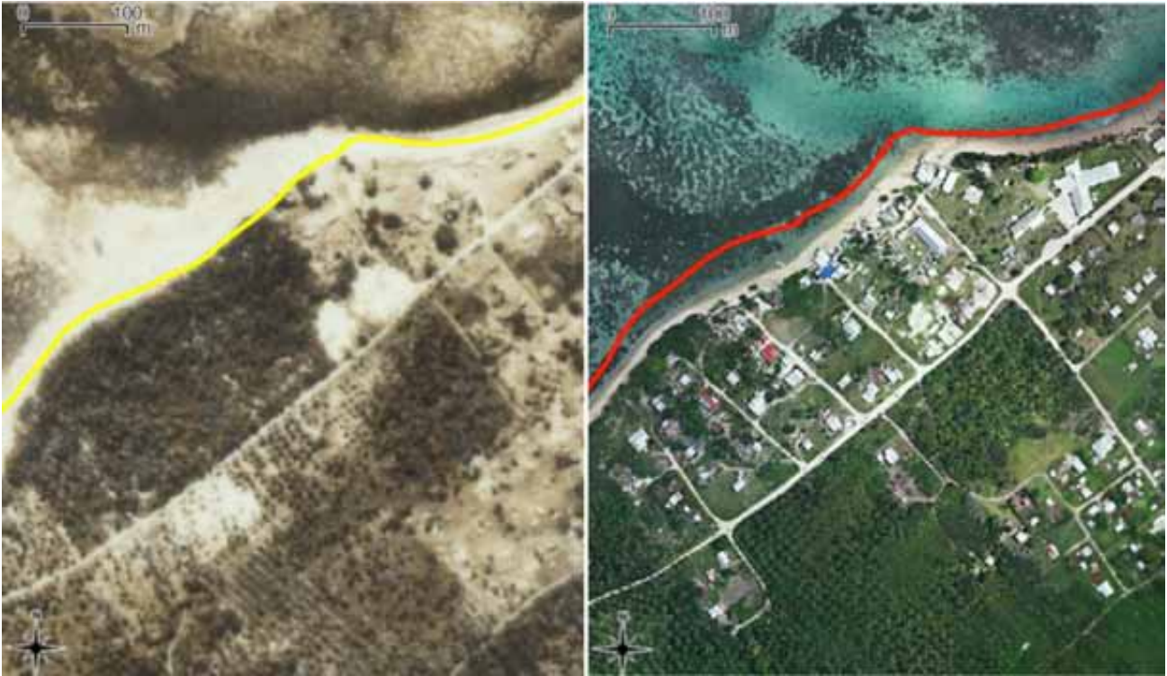
Figure 21: Left, Hihifo in 1968, with the 2011 shoreline superimposed. Right, Hihifo in 2011, with the 1968 coastline superimposed. Note the intense coastal development over the last four decades along this eroding shoreline.
