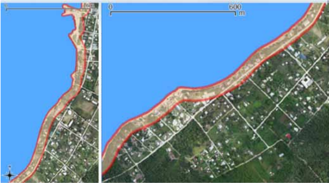
Figure 39: The space that would need to be taken for the construction of a rock revetment in (left) Pangai, and (right) Hihifo
