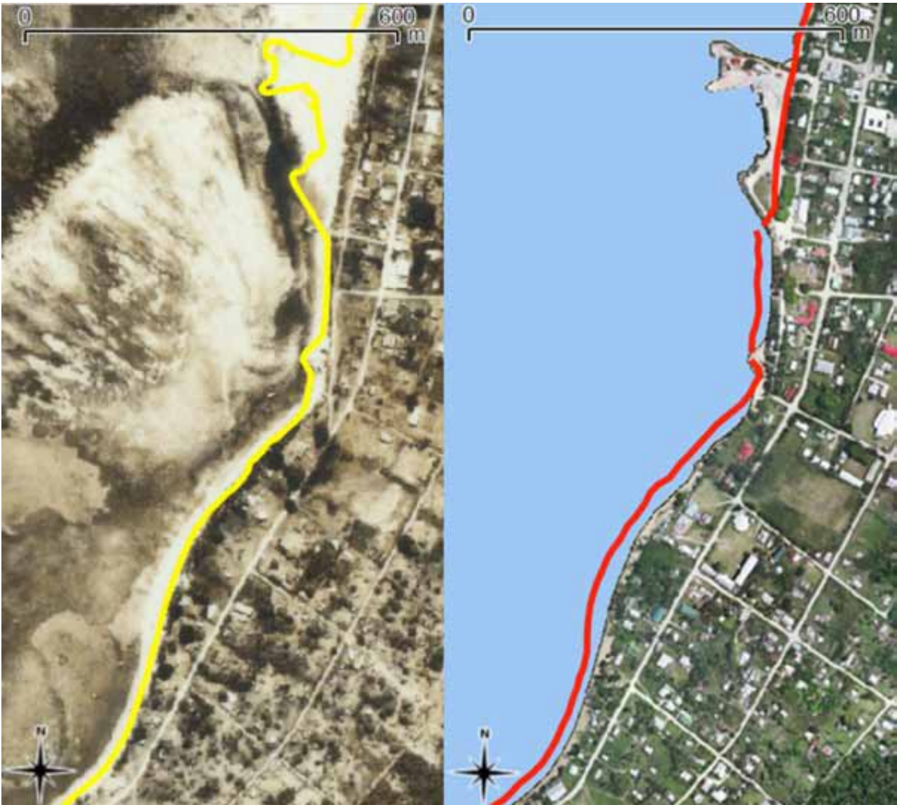
Figure 20: On the left, Pangai in 1968, with the 2011 shoreline superimposed. On the right, Pangai in 2011, with the 1968 shoreline superimposed. Note that the old piled jetty visible in the top third of the 1968 image was replaced by a stone causeway in 1982, and that the present Pangai Harbour, opened in 1996, is visible near the top of the 2011 image.
