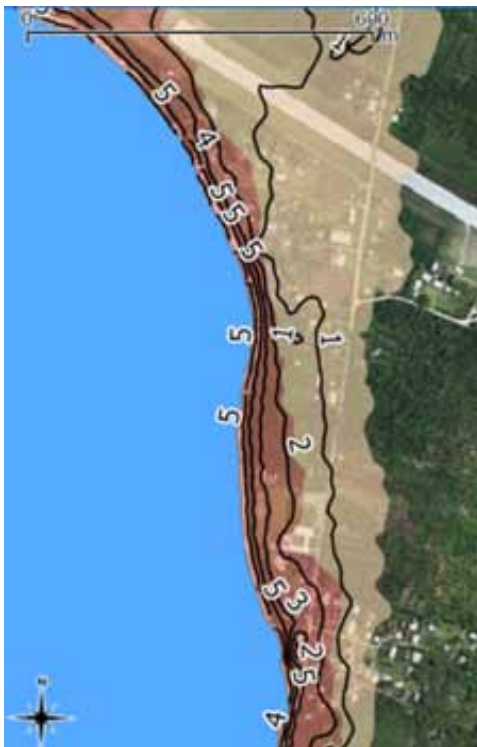
Figure 34: Koulo and Holopeka flood depths in metres, 2100, based on an intermediate–high sea-level rise scenario and severe tropical cyclone conditions (see text for details)
