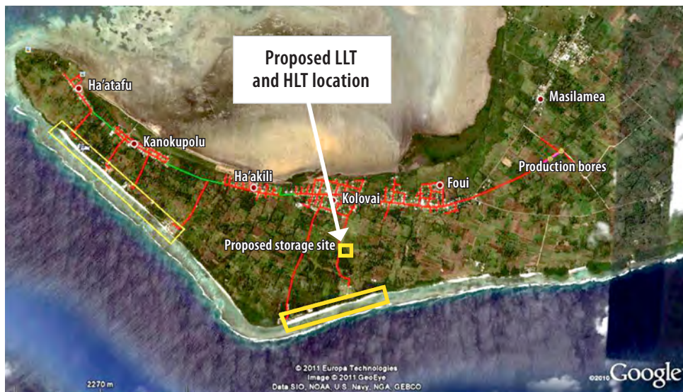
Figure 5. Layout of Hihifo pipe network and proposed location of high and low level tanks (source: Google Maps).
