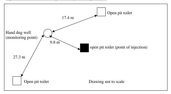
Figure 2.3 Plan View of Large Scale Dye Tracing, SITE 1
