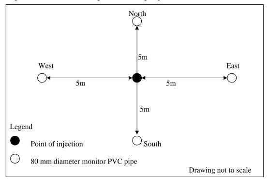
Figure 2.2: Plan View of Large Scale Tracing Experiment
