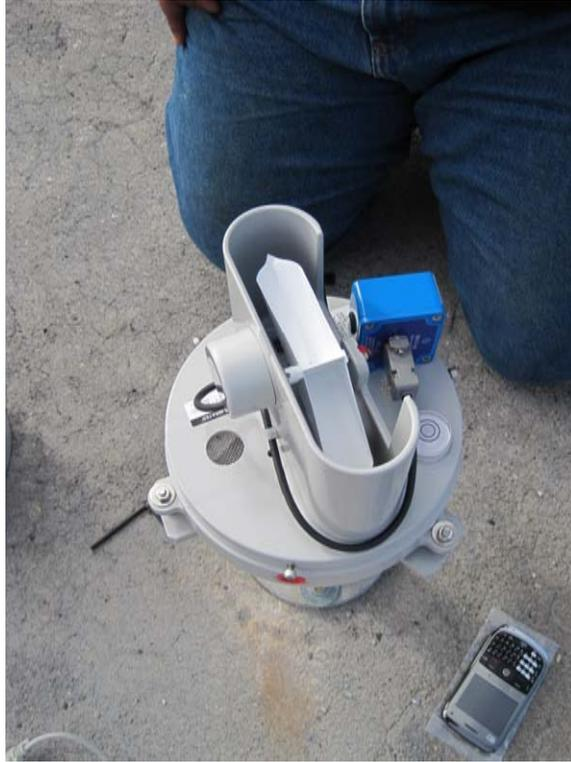
Figure 2: Gauge from above, without cover
