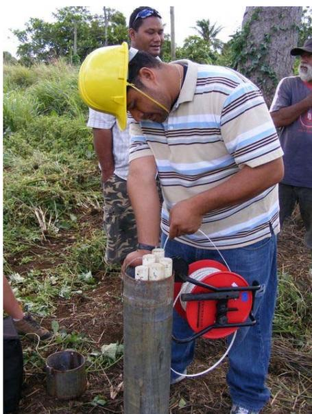
Water level measurement of monitoring bores
