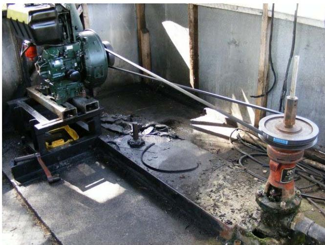
**Typical village well set up +ve displacement helical pump and Lister diesel motor**
