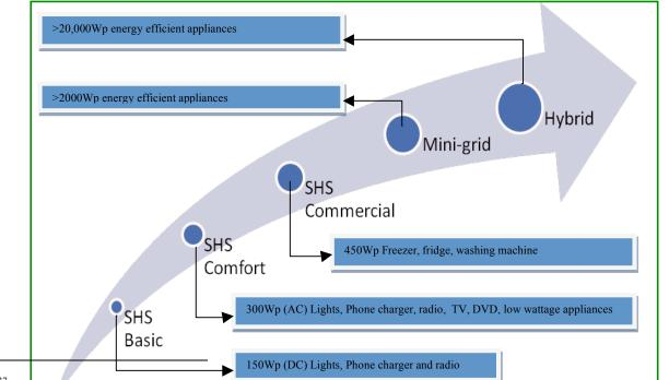
Figure 4.2: The Tiered Approach for Off-Grid Electricity Supply
