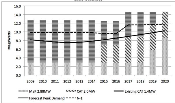
Figure 3.3: Installed Capacity on Tongatapu Required for the Median Forecast BAU Scenario
