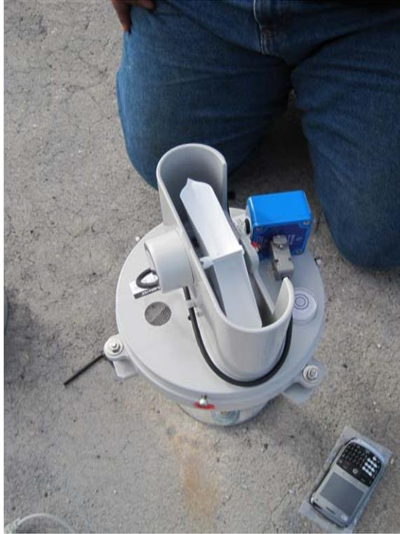
Figure 2: Gauge from above, without cover
